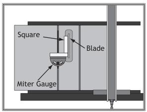
**Figure 108.** Checking the 90° miter gauge stop.
